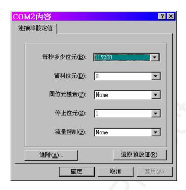
After settling down, connect our specific RS232 cable and press the 'call' icon of 'Hyper Terminal' program. After this, press 'Enter' key, if an '>' symbol come up, that means the unit is ready to accept commands for computer.
